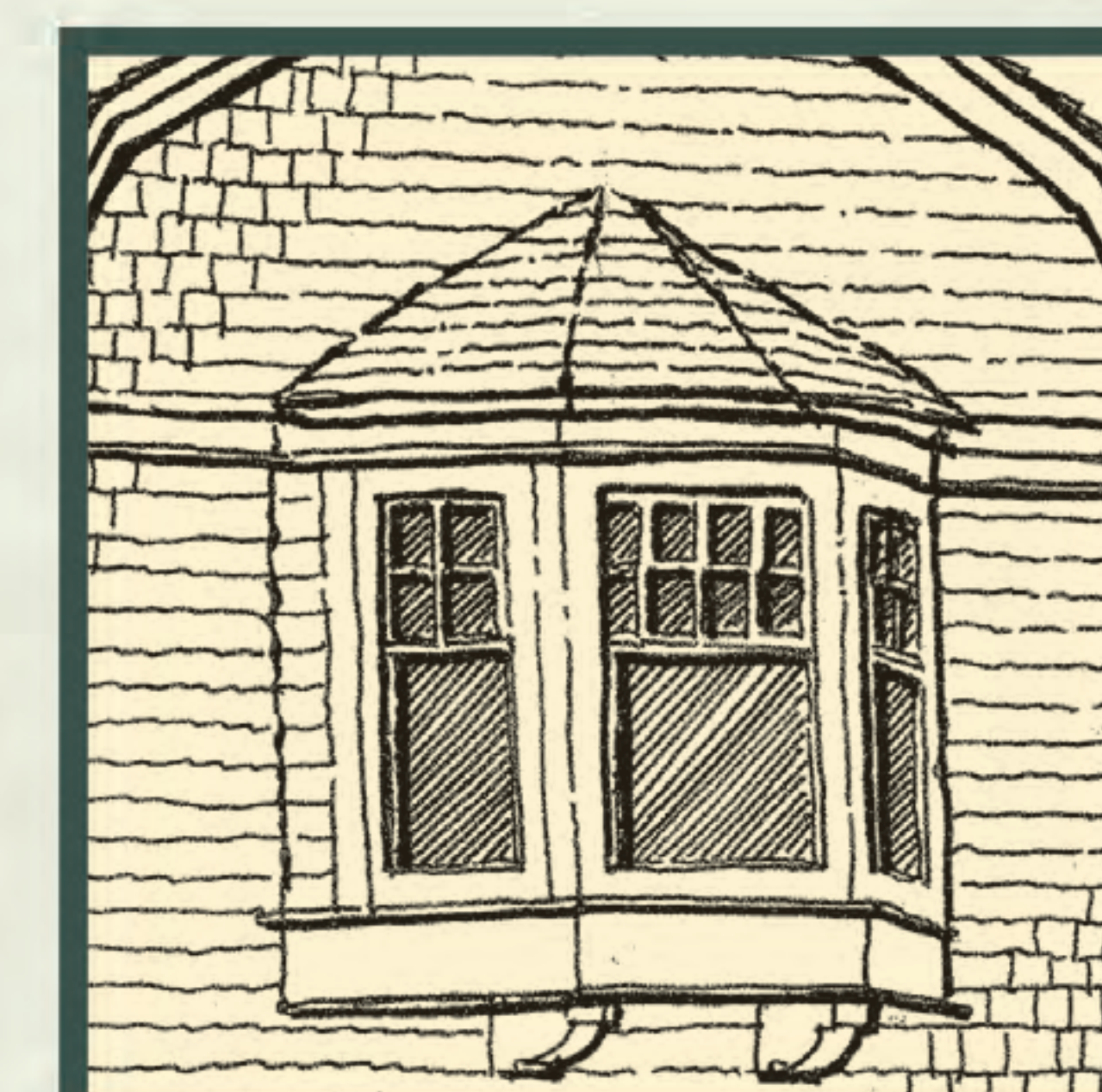
Bay window projection supported by corbels
